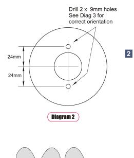
When drilling holes align cutter blades with propeller blades as shown. Drill two 9mm (3/8") diameter holes 5.5mm deep in the front face of the propeller boss as shown in Diagram 2.
