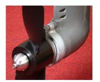
Refit the modified propeller (see instructions below) The heads of the two driving screws in the rotating cutter must engage in the two new holes in the propeller boss.
