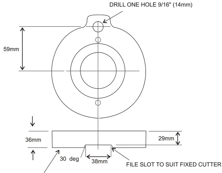
THE ANODE IS 40mm THICK AS STANDARD M/C 4mm OFF THIS FACE. ALSO BORE OUT 88mm BY 14mm DEEP
